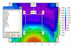
Finally, here is the result of using *Define Boundary* to remove triangles from the opening:
