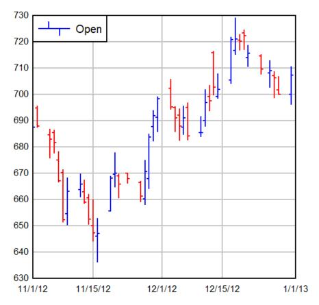
Tick mark length (and visibility) are a function of line width, extents, and plot size.
