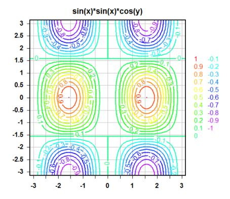
To switch to a 3D view, switch to shaded bands rather than contour lines, change the number of contour intervals or the upper and lower limits of those contours, and/or change the color scheme used for the contours, select *Options*><u>Contour Options</u>. The settings used for the example plot are shown here:
