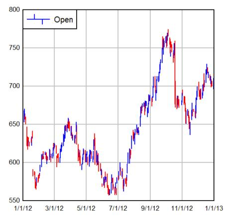
You'll note that the Open and Close tick marks aren't visible in this case. That's due to a combination of the <u>line width</u> used and the <u>extents of the plot</u>. Tick marks are always drawn 1/2 unit (normally 1/2 day) long, so if the days are spaced too closely **and** the line width is too large, the tick marks won't be visible. If you zoom in or use <u>Options>Extents/Intervals/Size</u> to isolate on the last 2 months of 2012, you should get something similar to this:
