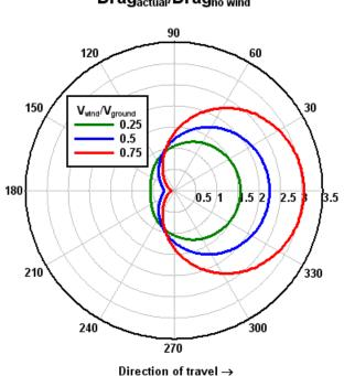
Relative Drag Force for a Spherical Object Drag<sub>actual</sub>/Drag<sub>no wind</sub>
