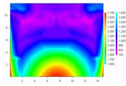
depicts peak pressure measurements across the face of a wall with an opening in the center of the wall. No gages were located within the opening, so the plot is at best misleading. If you use the *Contour Options* command to turn on the triangle borders then the opening location becomes more apparent:
