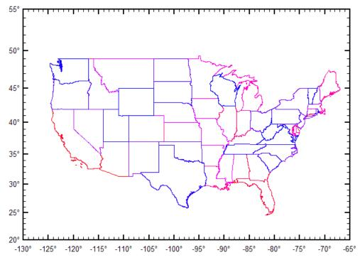
The vertical axis with this scaling is increasingly stretched out at higher latitudes. This scaling was originally made popular by its ability to represent lines of constant true bearing as straight line segments.
