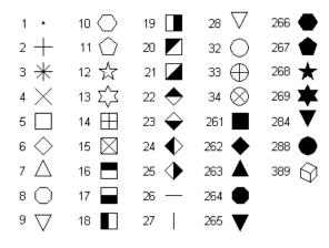
Symbols 28 and 284 are identical to symbols 9 and 265, respectively, with the exception of vertical alignment. Symbols 9 and 265 are placed such that the geometric center of the triangle is at the data point. Symbols 28 and 284 are vertically aligned with symbols 7 and 263.
