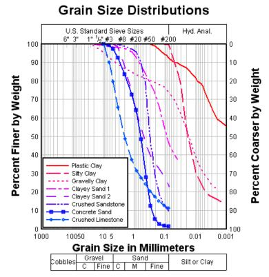
By default, the grain size plot is set up for grain sizes in millimeters. A U.S. Standard Sieve scale will be drawn at the top edge of the plot, and a scale showing the range in size of common engineering materials is drawn below the X axis. These features require that the units of the grain sizes be known. The units may be changed with the <u>Grain Size Options</u> menu command.
