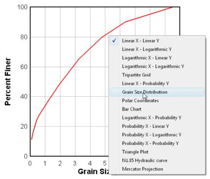
Alternatively, select Linear/Log Scaling>Grain Size Distribution on the Options menu. In either case this action will result in a grain size distribution plot with default settings:
