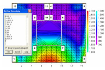
Finally, here is the result of using *Define Borders* to remove triangles from the opening:
