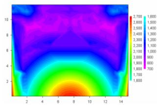
depicts peak pressure measurements across the face of a wall with an opening in the center of the wall. No gages were located within the opening, so the plot is at best misleading. If you use the *Contour Options* command to turn on the triangle borders then the opening location becomes more apparent:
